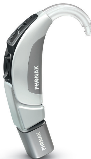
A hearing aid with an ear-level receiver connected by a direct input shoe.
